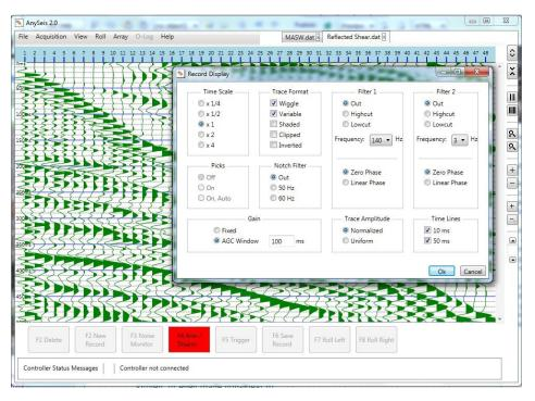
Data is displayed on a laptop computer. The acquisition and display parameters are controlled by the laptop, which also stores the data on the internal disk in a standard SEG format. Data can be archived on external media.
