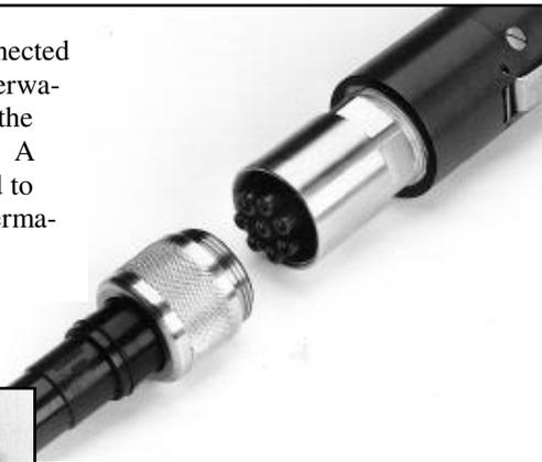
**Big Hole Adaptor:** An optional mechanical arm and pressure foot (shown here on the BHG-2) can be substituted for the spring to clamp the tool in large diameter boreholes. Conversion is easily done by the user in minutes. Multiple arms provide for various diameter holes. Largest arm extends diameter up to 480 mm (19 inches). When retracted, will fit inside a 75-mm (3-inch) diameter borehole.
