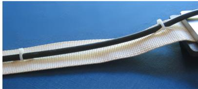
When land streamers are towed on rough ground with long geophone intervals, stations can tip over. In that case, attach the anti-rotation wing supplied with the system to add stability. KCL or equivalent connectors (as shown here) are preferred, but Mueller clips and split-ring takeouts are acceptable.
