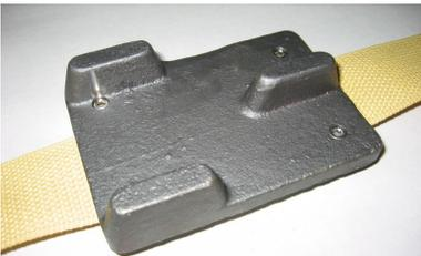
The tripod support provides stability, even if the ground surface has loose material, so the sensor will respond properly to ground vibrations. The legs will tend to plow into soft ground for better coupling.
