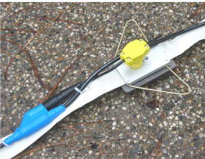
KCL or equivalent connectors (as shown here) are preferred, but Mueller clips and split-ring takeouts are acceptable.
